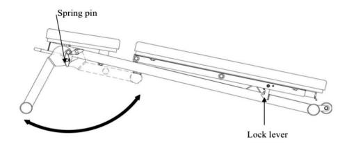
Pull spring pin to unfold or fold leg. Make sure hands are clear of pivot area. Make sure spring pin is fully engaged in locking holes after each adjustment.
