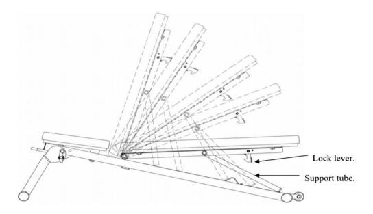
Swivel lock lever under pad to release back pad. Raise the head end of the pad so the free end of the support tube slips into a slot for a desired position. Before use, make sure the support tube is secure in a slot.
